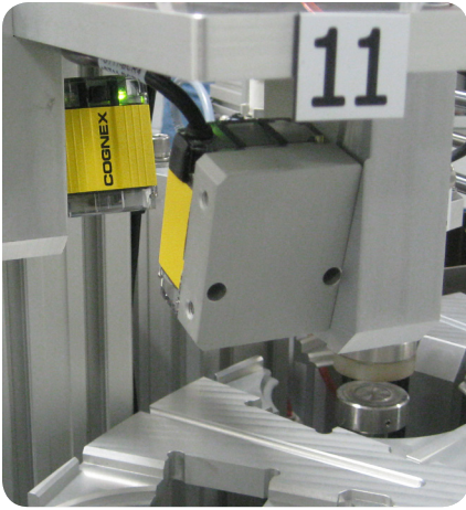
At the start of the returns process, the Netflix mailers are loaded onto the first of two rotating carousels. Each mailer is placed in a nest and then rotated under the second station where it is checked for thickness (no disc, one disc or two discs).
