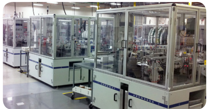
ARRM3600 units on the floor of the Netflix DVD returns facility. Each ARRM3600 inspection station can perform barcode reading and inspection tasks for 3,600 mailers per hour.
